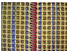
KEVLAR® SANDWICH JOINT : With PEEK spiral
